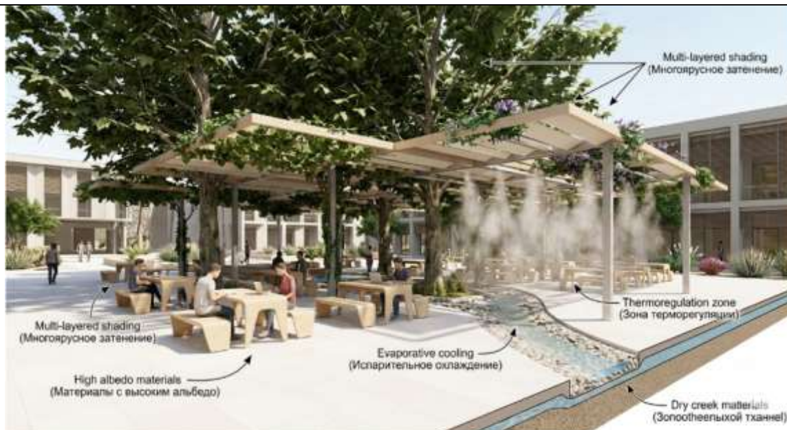
Figure 2. Biophilic adaptation strategies and microclimatic landscape design for arid regions: Integration of multi-layered shading systems and evaporative cooling in educational environments.
