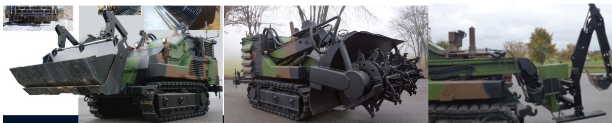
7-rasm. SDZ robotiga o‘rnatilgan ishchi organlari: buldozer, mina trali, ekskavator
