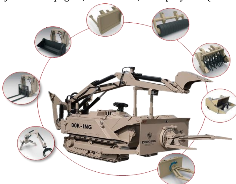
3-rasm. MV-4 roboti va uning almashtiriladigan ishchi organlari
