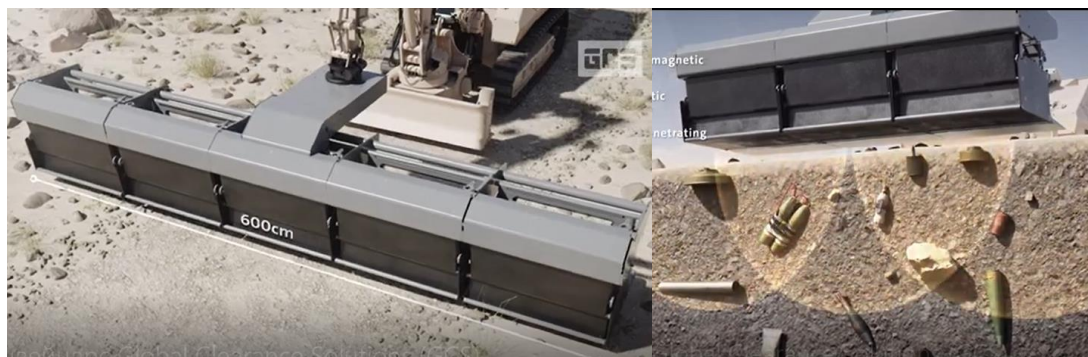
5-rasm. GCS-200 robotining minaizlagichi
