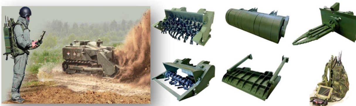
2-rasm. URAN-6 roboti va uning osma ishchi organlari
